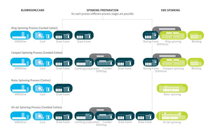
Fig. 19: Examples for complete manufacturing processes of the Com4 yarns
