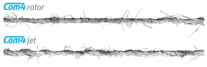
Fig. 12: Com4rotor and Com4jet yarn
